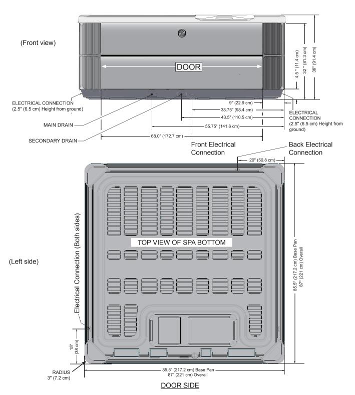
**NOTE: WATKINS WELLNESS** recommends that the **ARIA** be installed on a minimum 10 cm (4") thick reinforced concrete pad or a deck that is able to withstand more than 595 kg/m $^2$  (125 lbs. per square foot).
