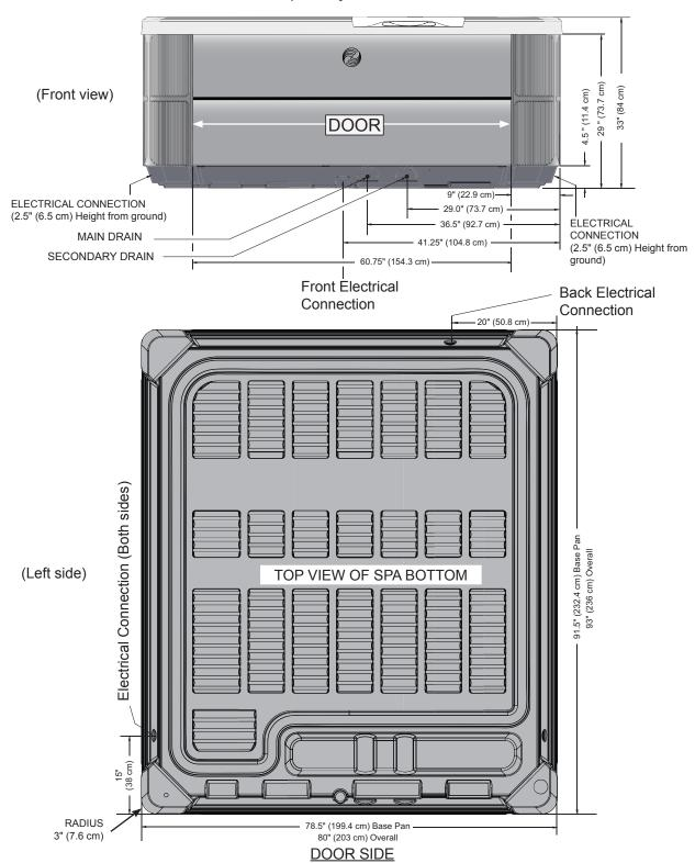
**NOTE: WATKINS WELLNESS** recommends that the **SOVEREIGN** be installed on a minimum 10 cm (4") thick reinforced concrete pad or a deck that is able to withstand more than 555 kg/m² (115 lbs. per square foot).
