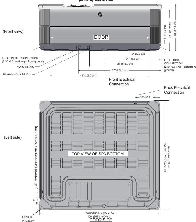
NOTE: WATKINS WELLNESS requires that the ENVOY be installed on a minimum 10 cm (4") thick reinforced concrete pad or a deck that is able to withstand more than 570 kg/m² (120 lbs. per square foot).
