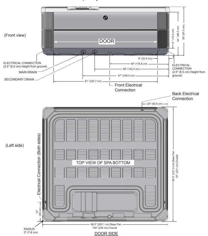
**NOTE: WATKINS WELLNESS** requires that the **GRANDEE** be installed on a minimum 10 cm (4") thick reinforced concrete pad or a deck that is able to withstand more than 605 kg/m² (125 lbs. per square foot).
