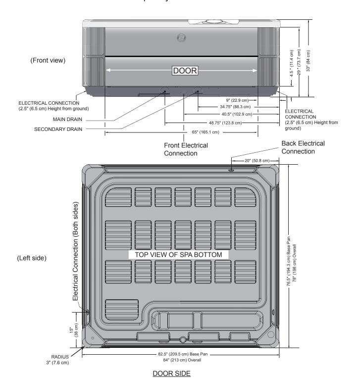
**NOTE: WATKINS WELLNESS** recommends that the **PRODIGY** be installed on a minimum 10 cm (4") thick reinforced concrete pad or a deck that is able to withstand more than  $595 \text{ kg/m}^2$  (125 lbs. per square foot).
