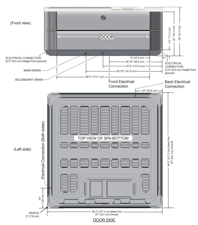
**NOTE: WATKINS WELLNESS** recommends that the **VANGUARD** be installed on a minimum 10 cm (4") thick reinforced concrete pad or a deck that is able to withstand more than 630 kg/m² (130 lbs. per square foot).
