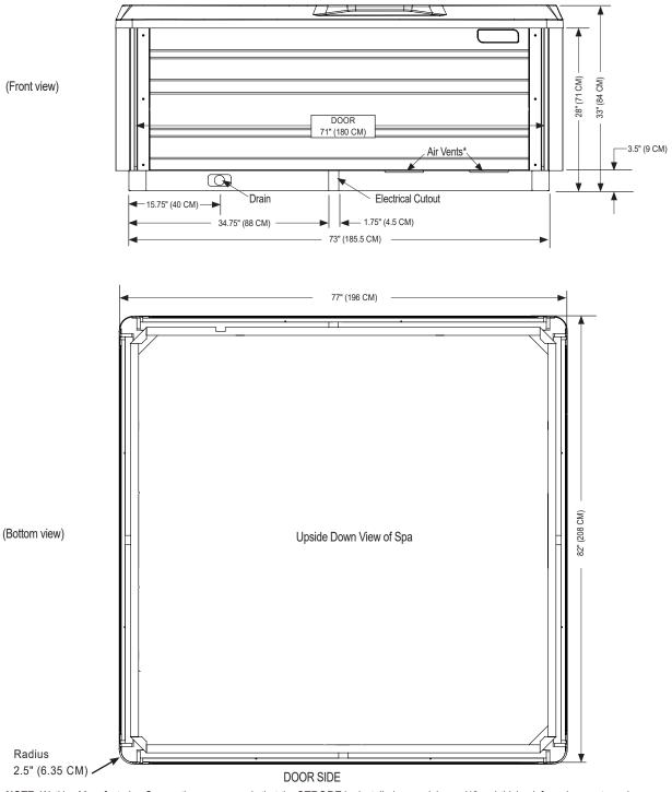
**NOTE:** Watkins Manufacturing Corporation recommends that the **STROBE** be installed on a minimum (10 cm) thick reinforced concrete pad or structurally sound deck able to support the "dead weight" found on the spa specification page.
