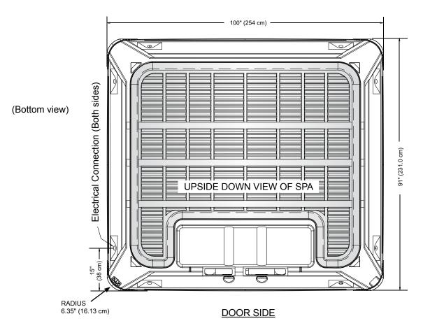
**NOTE: WATKINS WELLNESS** requires that the **GRANDEE** be installed on a minimum 10 cm (4") thick reinforced concrete pad or a deck that is able to withstand more than 555 kg/m² (125 lbs. per square foot).
