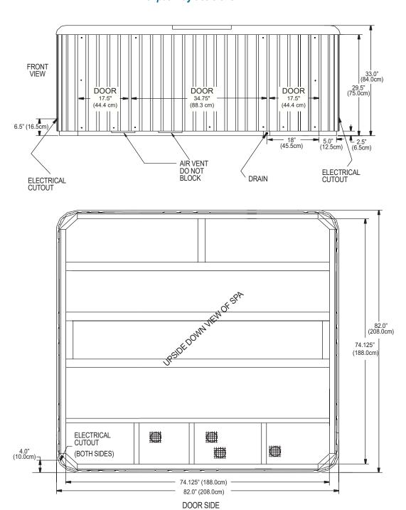
**NOTE:** Watkins Manufacturing Corporation recommends that the **PROPEL** be installed on a minimum (10 cm) thick reinforced concrete pad or structurally sound deck able to support the "dead weight" found on the spa specification page.
