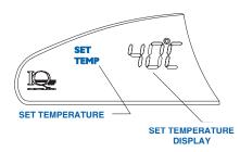
To display the set temperature of the spa, press the TEMP Plus (+) button. The set temperature will be displayed, unless the spa is locked (in which case the word SPA is displayed with the lock symbol). The set temperature display will automatically shut off after 30 seconds.
