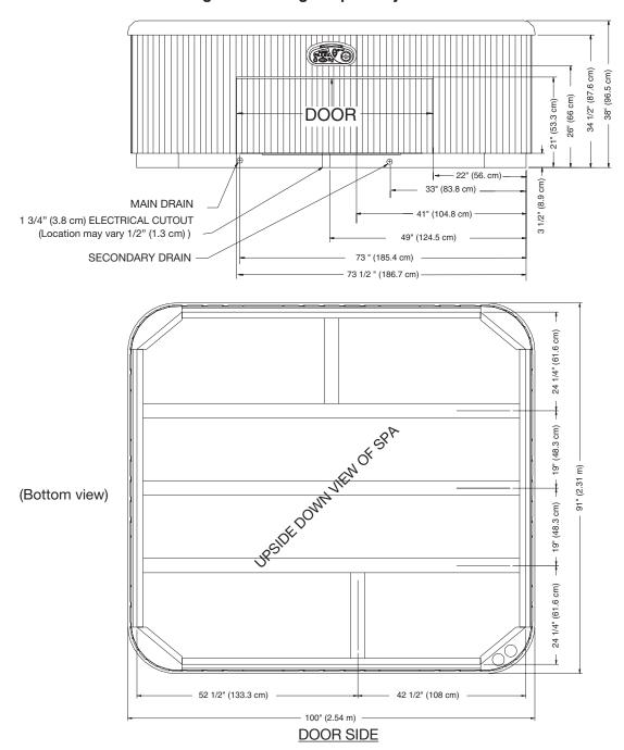
**NOTE:** Watkins Manufacturing Corporation requires that the *Grandee* be installed on a minimum 10 cm (4") thick reinforced concrete pad or a deck that is able to withstand more than 555 kg/m<sup>2</sup> (115 lbs. per square foot).
