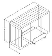
Next, contact your dealer to find the height and width added by the delivery cart which the dealer will use to deliver your new spa. Use the height of the cart plus the dimension shown as H to determine the vertical clearance required to pass the spa and cart. Use the width of the cart, or dimension W, whichever is greater, to determine the maximum width of clearance necessary.
