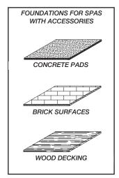
If you are purchasing a deck package or a gazebo with your spa, a solid foundation is mandatory. Placing them on any surface other than a single level pad could create problems with their installation. Pictured on the previous page are a few of the recommended surfaces.
